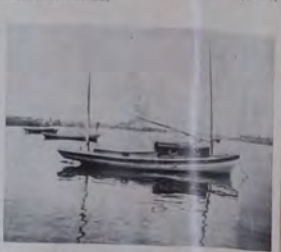
A comfortable cruiser adapted from an oyster skiff 27 ft. length, 7 ft. beam; cost $400
