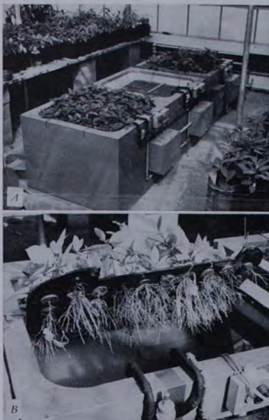
Fig. 1. A) Temperature-controlled tanks with avocado seedlings growing in aerated nutrient solution. The seedlings are supported by the rack shown in the middle tank. B) Healthy roots of avocado seedlings prior to inoculation. Note the cheesecloth bags with the inoculum.
